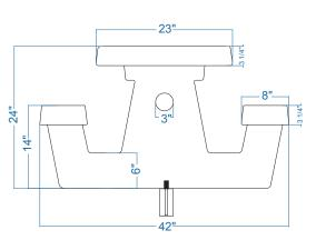
Threaded coil inserts and rods provided with table for mechanical attachment into 3" dia. Grout pocket on site by others.
