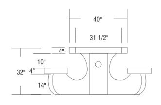
1. Concrete mix design to include a mixture of Portland Cement, name to the residue of mixture of Portland Certer water, coarse and fine aggregates, pure mineral oxide coloring agents (when applicable) to yield a minimum compressive strength of 5000 psi.
