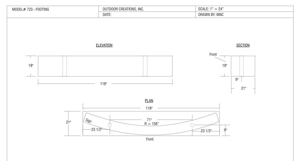
1. Cast (2) mounting thru holes (grout pockets) minimum diameter 3", in footing as shown.
